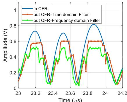
Fig. 6. Amplitude waveforms at CFR input and output with 15 optimizable coefficients.
