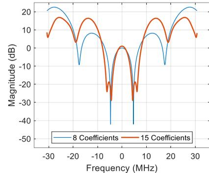
Fig. 5. Optimized FIR filter frequency responses.
