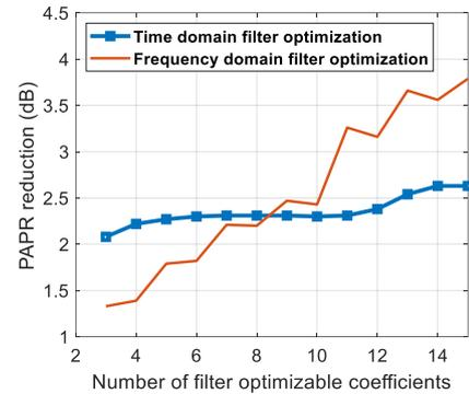
Fig. 4. PAPR reduction in function of the number of filter optimizable coefficients.
