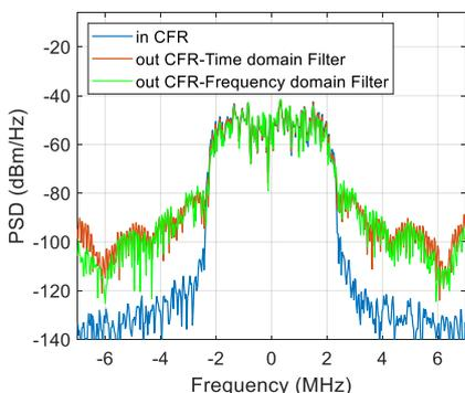
Fig. 7. Power spectral densities at CFR input and output with 15 coefficients.
