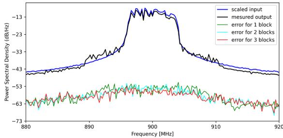
Fig. 6. Power Spectral Density (PSD) for measured input and output signals and modeled errors
