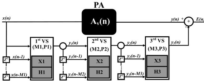
Fig. 1. Proposed model with three Volterra series in cascade
