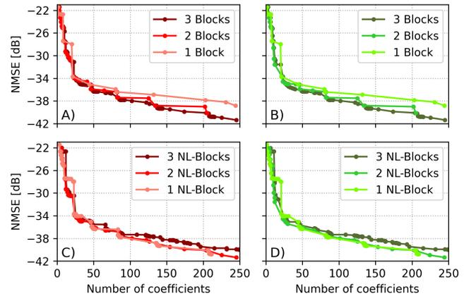
Fig. 4. NMSE curves. A) Traditional model and cascade derivations with two and three blocks (SLS parameter extraction). B) Optimized results from "A)". C) Three blocks cascade Volterra series for different numbers of nonlinear blocks into the scheme (SLS parameter extraction). D) Optimized results from "C)".
